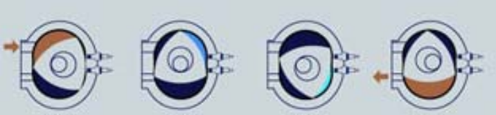
Intake Compression Explosion Exhaustion
