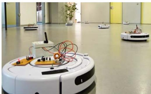
Figure 1: A robot swarm consisting of iRobot Roombas.
